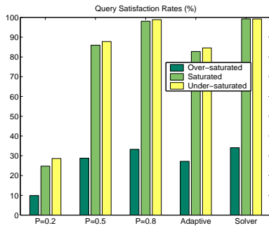
Figure 6: Query satisfaction rates (percent) for over-saturated, saturated, and under-saturated systems. 600 total grid nodes: 300 providers and 300 requesters self-organize into 60 neighborhoods of size ten each.
